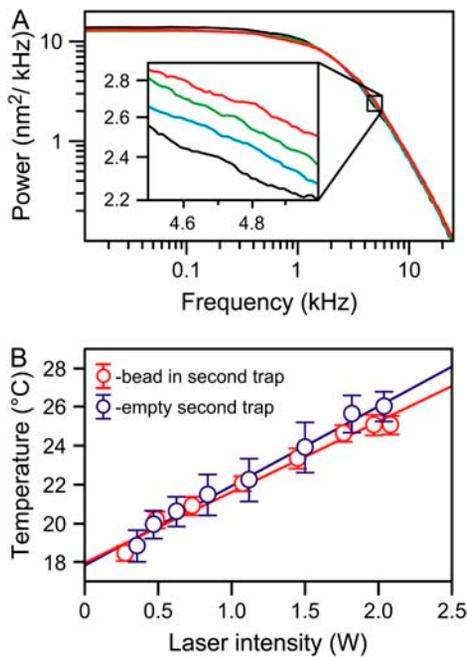
**FIGURE 1** (A) Power spectra for a bead held in an optical trap measured while the intensity of a second, nearby trap was modulated (laser intensities, 2.0 W, red; 1.4 W, green; 0.7 W, blue; 0.3 W, black). (B) Temperatures determined from fits to power spectra (mean  $\pm$  SE), plotted as a function of laser intensity.
